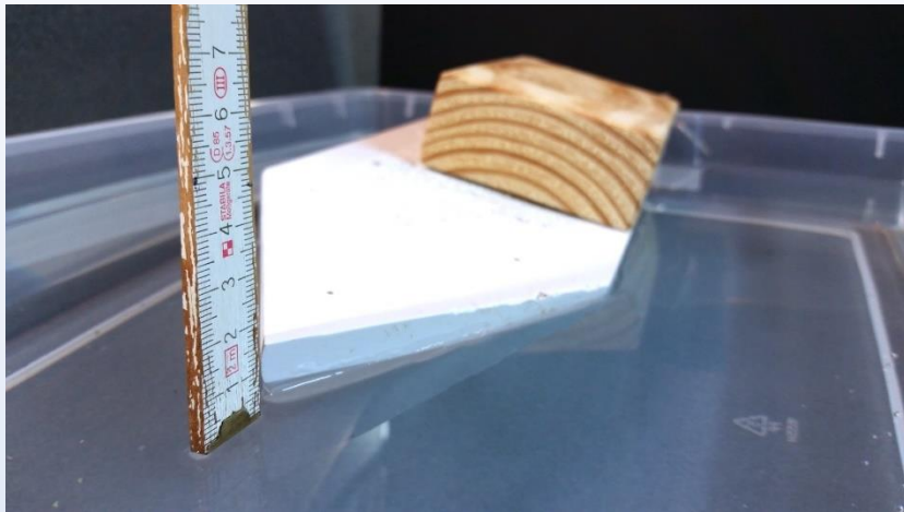
Bow waterline measurement with load shifted towards the port side from the center of the boat. (This boat: 14 mm)
