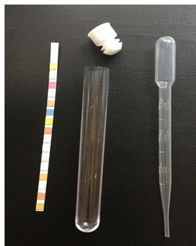
Figure 2. From left to right: test strip, test tube and cap, transfer pipet.
