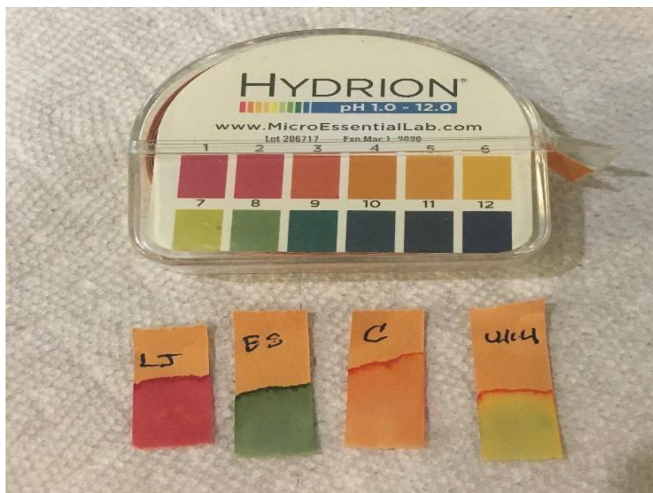
Figure 6. What pH values would you assign to each of these four test liquids? Compare the color to the pH color key. How do your results compare to the results provided in Figure 3?
