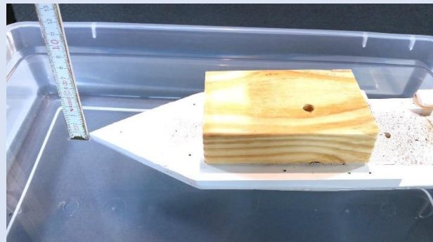
Waterline measurement at the bow with load two inches in the front. This boat: 4 mm.
